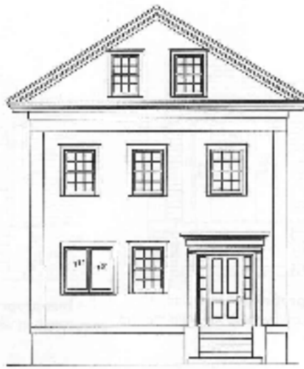
↑ Inappropriate Replacement single-pane casement window with enlarged opening. Missing drip caps.
