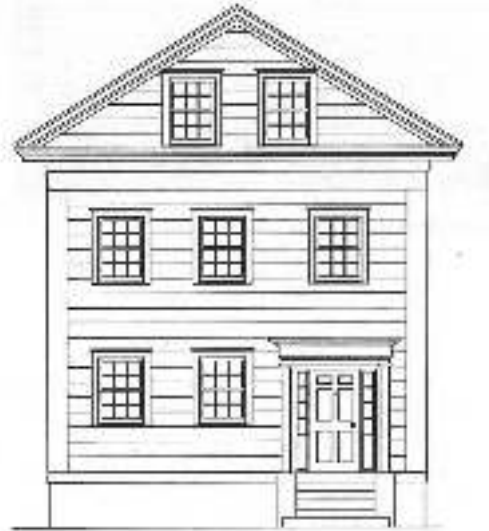
↑ Inappropriate Clapboards are too wide.
