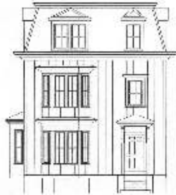
↑ Inappropriate Vertical siding
