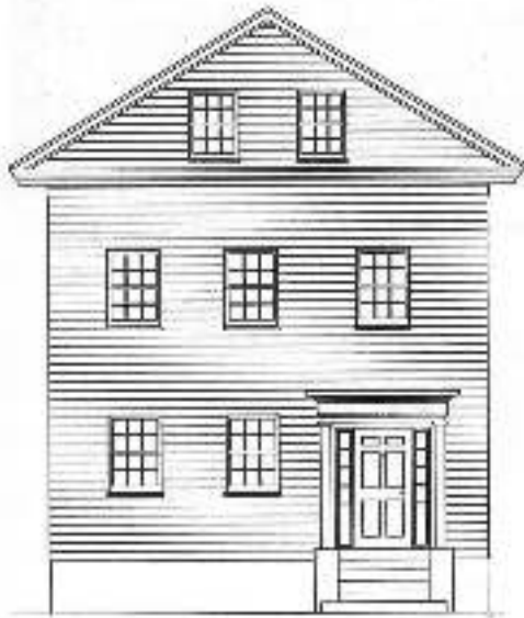
↑ Inappropriate Aluminum or vinyl siding. Loss of cornerboards, window trim and other details.
