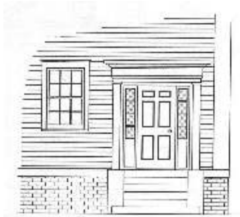
↑ Appropriate Original six-panel wooden door with sidelights.
