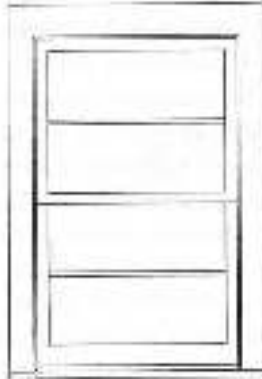
↑ Inappropriate Casement sash instead of double hung sash.
