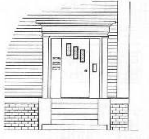
↑ Inappropriate Sidelights replaced by mailboxes and buzzers.
