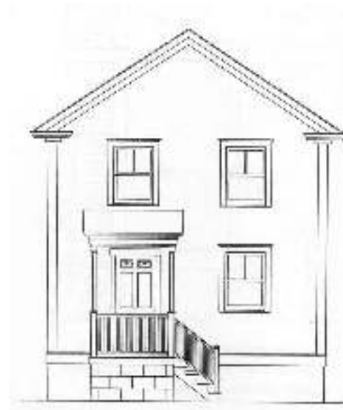
↑ Inappropriate Cinderblock porch base.
