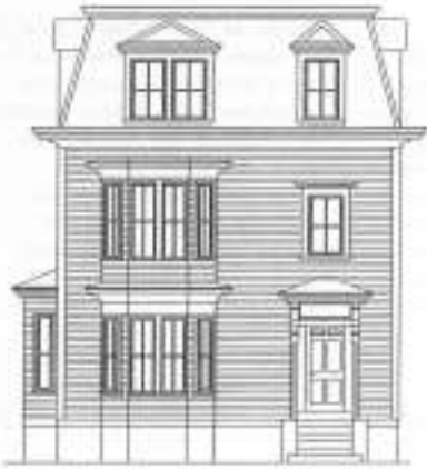
↑ Appropriate Original clapboards
